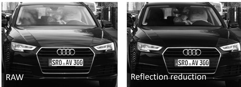
Figure 7: Reflection reduction by applying minimum signal of each calculation unit
