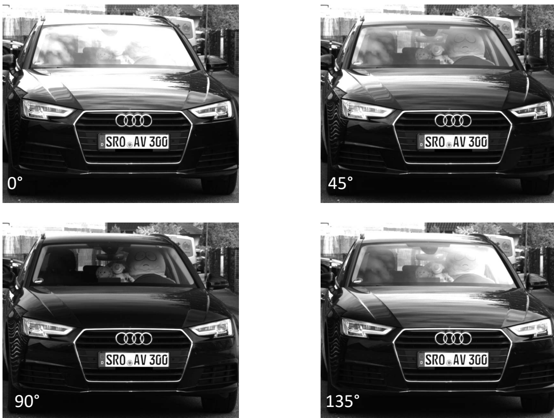
Figure 5: Polarization angle versus image brightness in sub-images
