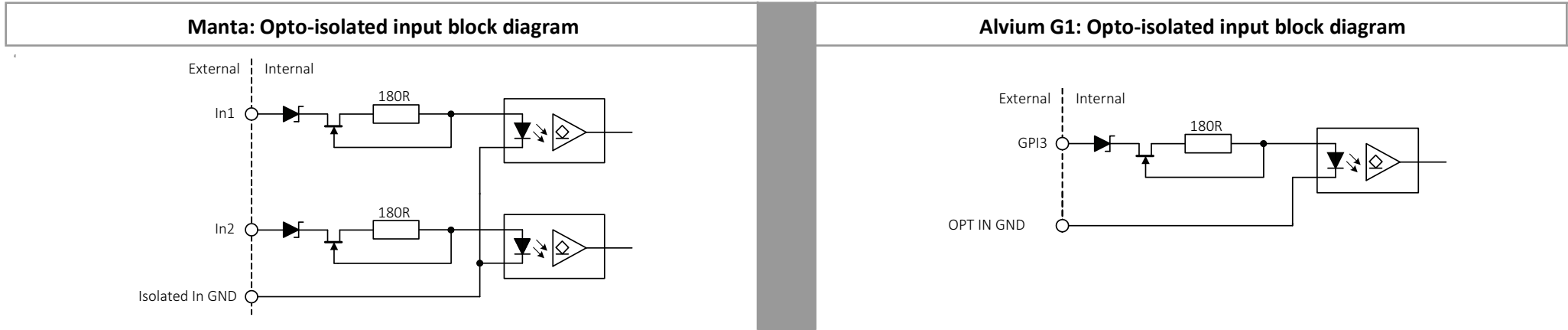
Figure 6: Opto-isolated input block diagram | Manta versus Alvium G1
